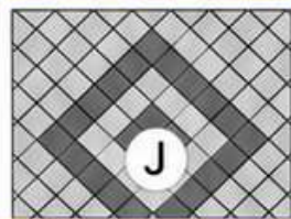
J 45° Stack Bond with contrasting diamond inlay
